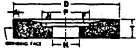
Type 23 — Wheel, relieved and recessed same side. Peripheral grinding wheel having one side straight or flat and the other side relieved to a recess.
