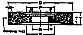
Type 25 — Wheel, relieved and recessed one side, relieved other side. Peripheral grinding wheel having one side relieved to a flat and the other side relieved to a recess.
